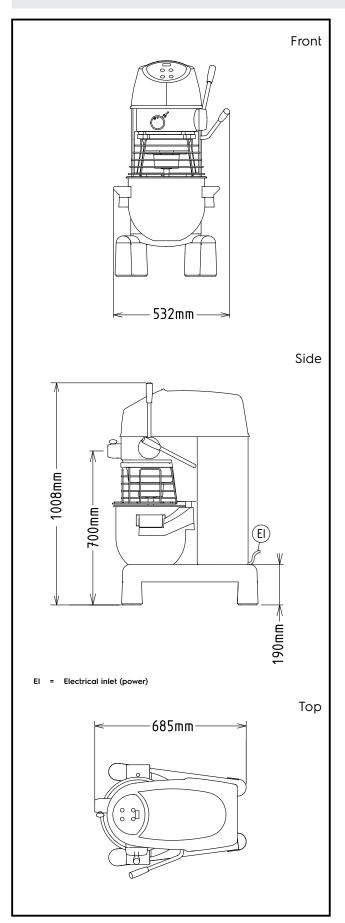
Electric Supply voltage: 208-230 V/1N ph/60 Hz Capacity: Performance (up to): Capacity: 20 litres **Key Information:** External dimensions, Width: 521 mm
